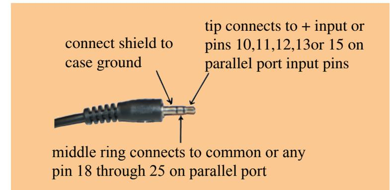
If your breakout board has a very large pull up resistor the probe will not work correctly wired this way, the LED on the probe will work but the signal will not be seen at the input. This is because the LED and .....Continued on back.....
