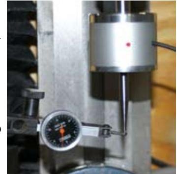
It is very easy to disassemble and repair, in case you have a crash. Just unscrew the top. I put it in a vice holding onto the probe tip to keep it from turning and hold the body in one hand to also keep that from turning. Then with the other hand unscrew the top cap from the body.
