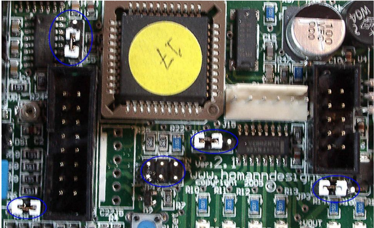
Figure 2.1 – Standard jumpering for use with RS-232
