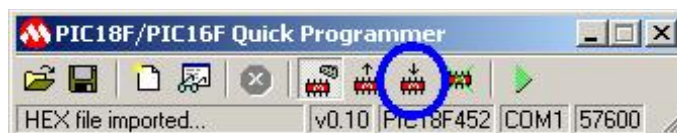
Figure 7.6 – Hex file loaded and the Write device icon
