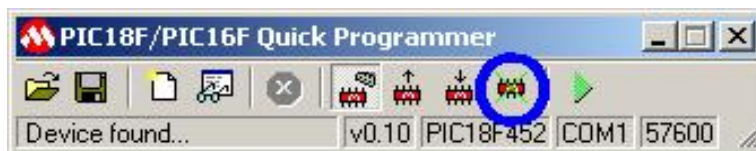
Figure 7.4 – PIC identified and the Erase icon
